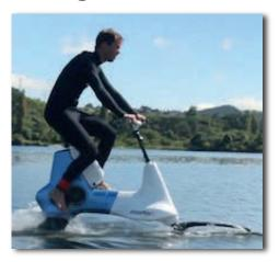
The *Manta5* hydrofoil bike promises to replicate the cycling experience on the water. Pedals connected to an electric motor power a propeller. The bike then glides on top of the water via a set of ski-like hydrofoils.
